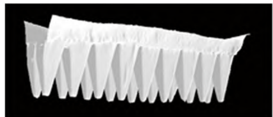
OCT检测3D模型侧视图 Ultrasonic welding joint photo taken by OCT with 3D image.
